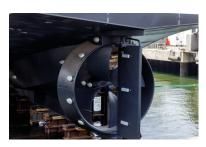
For the Shrimp Trawler this has resulted in an aft ship with enlarged propeller diameter.
