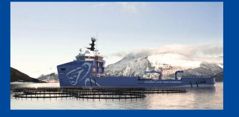
Damen has developed the concept of converting offshore vessels into live Well boats. An example of this is the Live Fish Carrier 8916. Offshore vessels are well-suited for modification for the aquaculture industry as a result of their behaviour.
