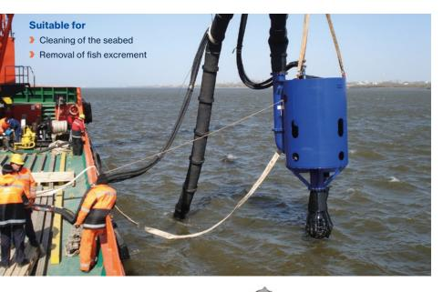
Damen offers high efficiency, wear resistant dredge pumps. Many different suction heads are available to fit any
