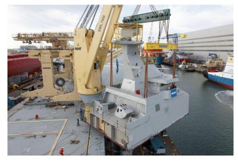
Damen builds its SIGMA corvette/frigate family to a standardised design that can be enlarged in a modular manner to meet different requirements. Pictured here at Damen is a pre-outfitted module for an Indonesian Navy SIGMA 10514 Martadinata-class frigate being delivered under Indonesia's Perusak Kawal Rudal (PKR) programme. (Damen Shipbuilding Group)
