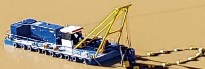
The Damen DOP pump is also available with an electrical drive. The compact and efficient electric motor directly drives the pump shaft. This clean and silent technology is especially fit for environmentally sensitive or residential areas.
