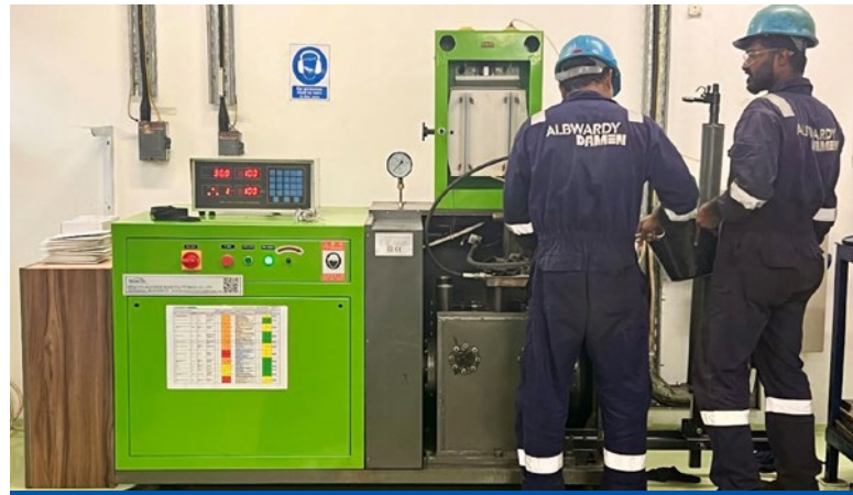
Fuel pumps are being bench tested in workshop prior to onboard installation
