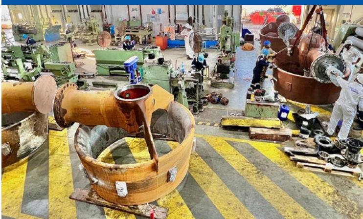
Workshop spaces are fully occupied with various thrusters for overhauling
