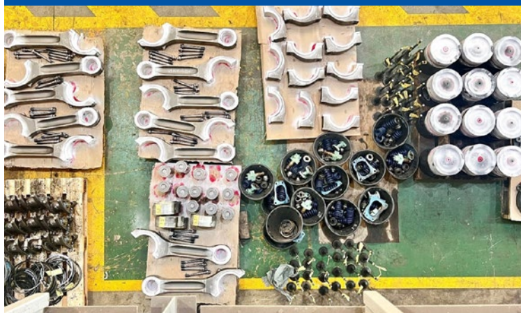
Engine components are disassembled and kept after inspection
