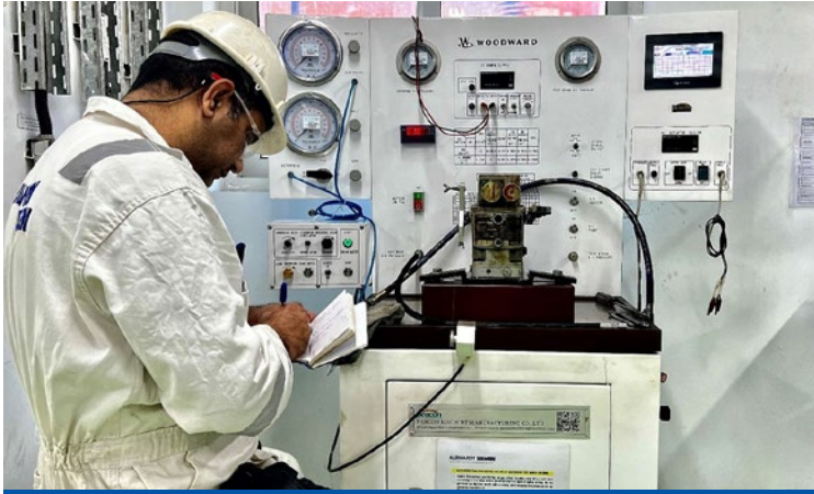
Governor and FO pump specialist is being engaged in testing of governor (before overhaul)
