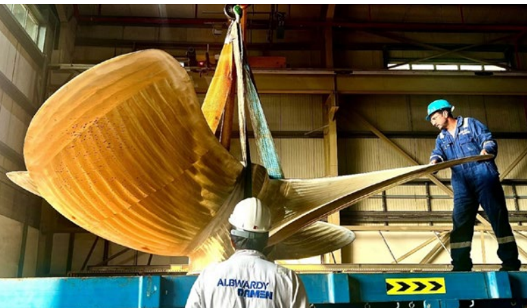
6-ton weighted propeller is dispatching after repair
