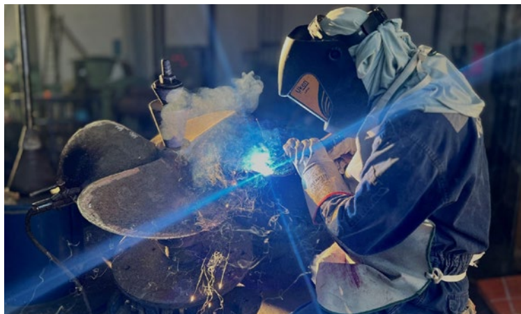
Small diameter propeller is being reconditioned
