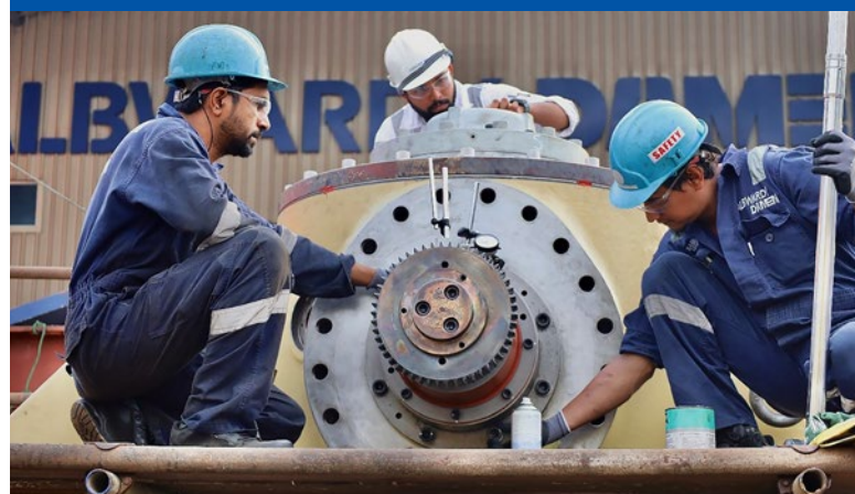
OEM Engineer and Mechanical team engaged in Niigata ZP-41 thruster assemble back
