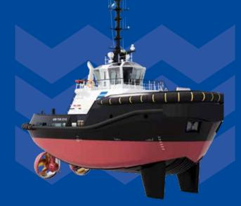
Paramount for safe operations are good, predictable handling characteristics, along with extreme stability. This comes courtesy of the vessel's low profile, wide-beam combination with a patented Twin Fin skeg design.
