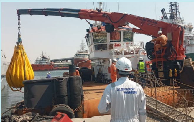
Re-calibrating LMI on Heila crane HLRM 200 4SL at Albwardy Damen yard Sharjah Hamariya Vessel: Cybi Island . Client: Holyhead Towing Co. Ltd
