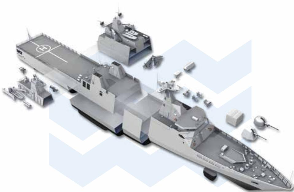
Building standard vessels in a series gives our clients fast access to proven, reliable technology. Our standard designs can be tailored to individual needs via modular construction, so our clients receive the ideal vessel, whatever challenge they are facing. Standard designs can always be equipped with various options to suit specific tasks.
