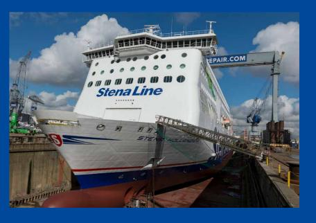
Damen Shiprepair Rotterdam carried out the docking of the 240 metre freight and passenger ferry *Stena Hollandica*. A key part of the docking was the installation of scrubbers to reduce the emission of sulphur compounds and particulate matter from the vessel's engines. Owner Stena Line is in the process of installing scrubbers on their vessels as part of an initiative to reduce its overall environmental impact.
