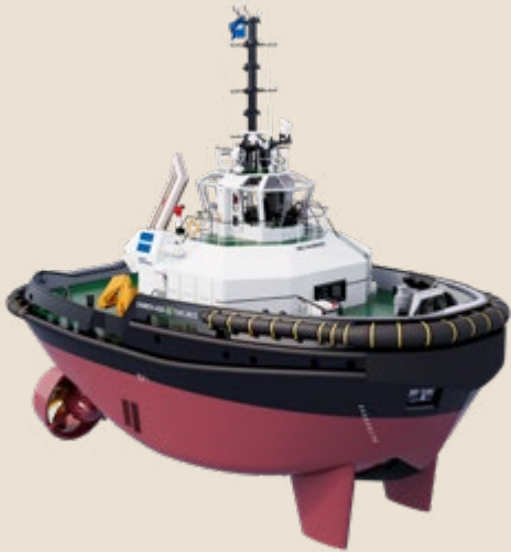
Our concept for an Azimuth Stern Drive 2613 Tug ...but on methanol.
