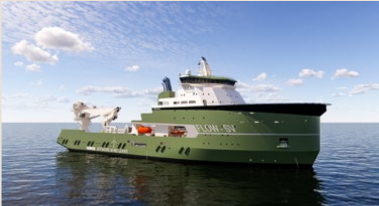
Our new concept for a Floating Offshore Wind Support Vessel. The Damen FLOW-SV 400 is specially designed to install ground tackles for offshore turbine floaters.
