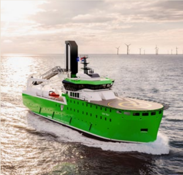
The 'cover model' of this edition. The Service Operations Vessel (SOV) 7017 is the smaller sister of the successful ASV 9020. This novel class of offshore wind support vessel has been named the SOV E. Our SOVs flourish in specific jobs; the vessels serve to provide hotel functions and stepless access onto offshore wind farms and oil & gas structures for technicians.
