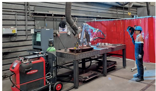
Figure 3: Welding cobot at Damen (Damen)
